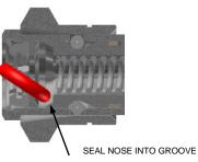
4. After nose of seal is in place, slowly press down on the back part (peak) of the seal using the knobbed end of pick.
