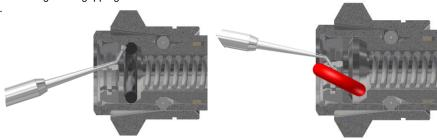
4. Using the knobbed end as a hook, dislodge the seal and pull it slowly out the connector throat.
