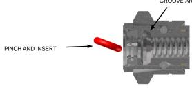
3. The knobbed end of the pick will assist in positioning the seal nose into the groove. This starting position is important for successful installation of the seal.
