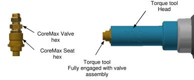
3. With the tool fully engaged with the CoreMax Valve/Seat assembly, squeeze the Trigger of the tool. The tool will spin the Core Valve into the seat until 8 ft/lbs. of Torque is achieved at a speed of 200 RPM's (max). Once the proper torque is achieved the torque tool will shut off.
