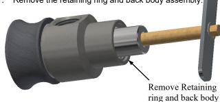
2. Remove the shaft clip. Then remove the shaft from the back body.
