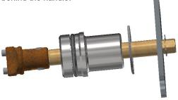
3. Insert the shaft assembly into the body of the connector.
