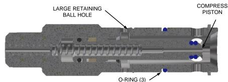
8. Install the sleeve friction o-ring(3) into groove on outside of the body(2).
