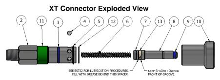
Please thoroughly read the instructions prior to rebuilding the XT Connector. If you do not understand instructions, or if components are missing, call *FasTest* before rebuilding connector.
