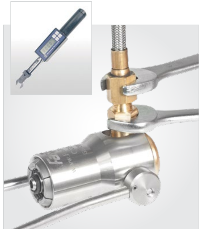
Figure 1. Torque to maximum 15 ft-lb
