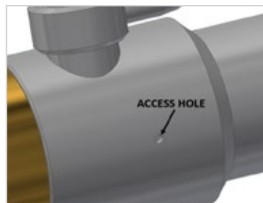
Figure 16. Safety pin area for WOB style connector shown. Pin is in the area beneath access hole.
