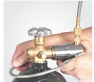
Figure 7b. Use minimal force on bail and handle
