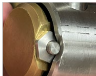
Figure 15. Example of a bad or damaged safety pin. When the pin is bent it will not retract. There is a noticeable indentation on the sleeve from contact with pin. The handle is also bent from forcing actuation while the pin is protruding out
