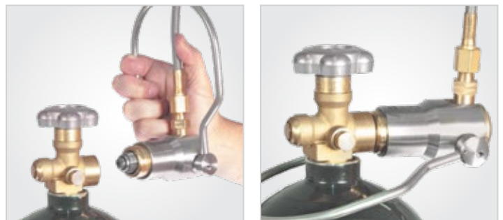
Figure 4c - 4d. Align CGA 580/590 connector tight and square against valve with no visible gap to avoid damage to the sealing surface
