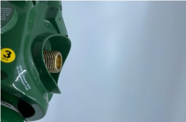
Figure 19. Make sure valve is clean and undamaged with room for connection
