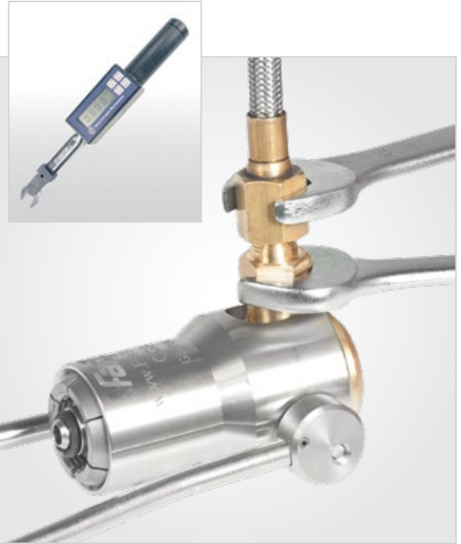
Figure 1. Torque to maximum 15 ft-lb
