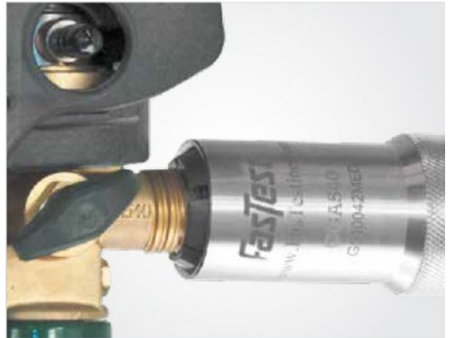
Figure 25. Note excess threads.
