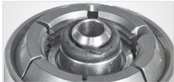
Figure 28. An example of a bad O-ring main seal
