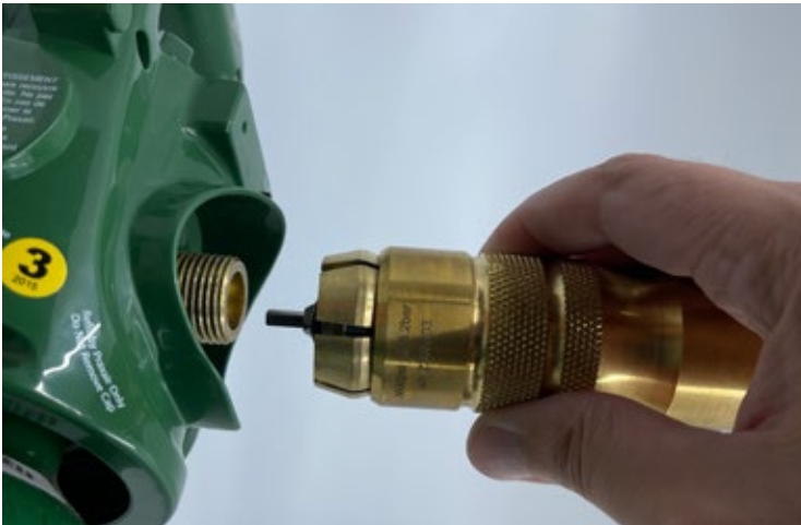
Figure 20. Align connector with valve and push on gripping the outer sleeve
