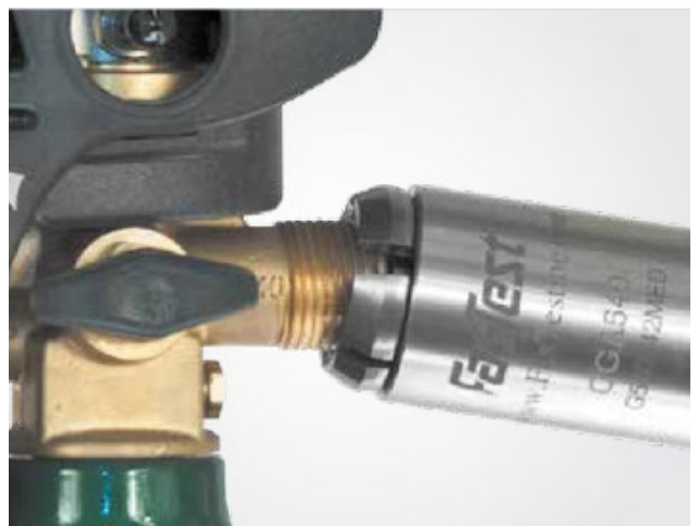
Figure 26. Connector loose and sleeve not forward.
