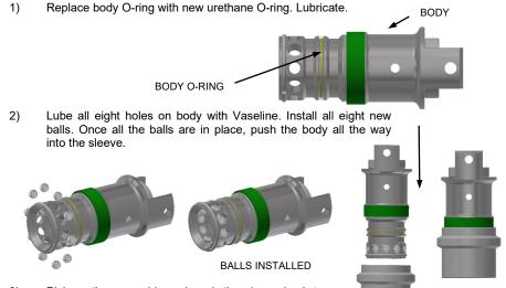
Pick up the assembly and push the sleeve back to expose the snap ring groove. Insert the new snap ring into its groove.
