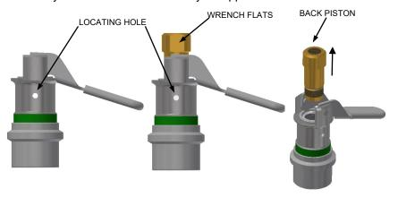
2) Once the brass back piston is removed, remove the spring and poppet assembly.
