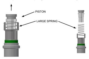
5) Slide sleeve back to expose snap ring, remove the snap ring on the front of the main body assembly and slide off the sleeve. Note the balls will be free so place in a catch basin.
