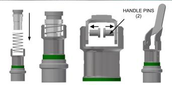
NOTE: 1/4" SIZE (KA04xx) REQUIRES HANDLE ORIENTATION. THICK SIDE OF HANDLE MATCHES TO THICK SIDE OF BODY TAB AS SHOWN. (No special orientation on 3/8" size.)
