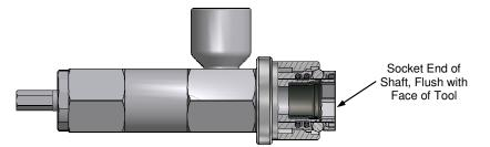
4. Place the Insertion Tool socket onto the Core at the top of the Core Loading Tool.
