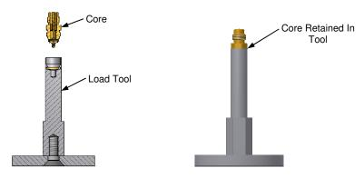
Core Insertion Tool (SCFT10) preparation. Pull the sleeve back and hold, then push the shaft in all the way. The socket end of shaft will almost be flush with the end of the tool.
