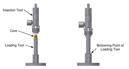
5. Push the Insertion Tool down until it contacts the bottom of the Loading Tool. You will feel the Insertion Tool engage at the bottom of the Loading Tool.
