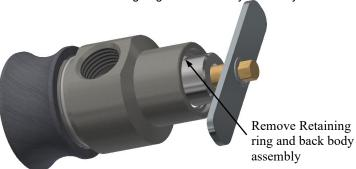
Remove the shaft clip. Then remove the shaft from the back body.
