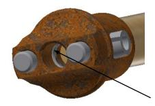
Remove and replace drive shaft seal
