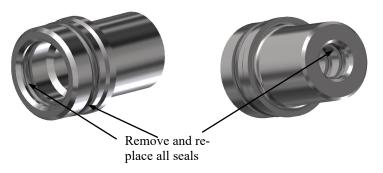
1. Remove and replace the small o-ring inside of the core driver head. Use a small screwdriver or pick. The seals are to be lubricated with refrigerant oil.
