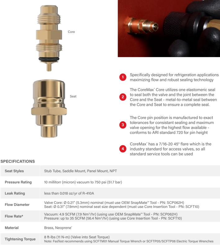
\*Flow rate indicated is through the valve core using the OEM SnapMate connector. Processing/flowing through the Seat only using the Core Insertion Tool will provide significantly more flow capacity.
