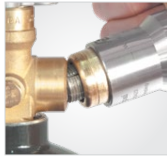
Figure 7c. Misaligned connection with internally threaded cylinder valve.
