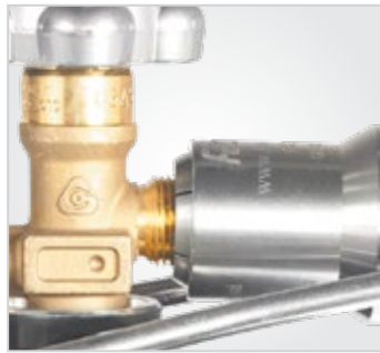
Figure 6d. Exposed threads indicating possible short connection on externally threaded cylinder valve.
