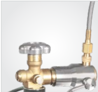
Figure 7a. Demonstrates good connection to valves with internal threads.
