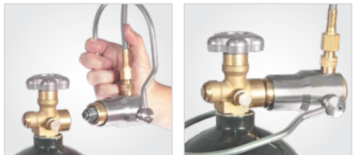
Figure 4c - 4d. Correct alignment and connection of connector for internally threaded valves. Note: align connector tight and square to valve face with no visible gap showing collet threads.
