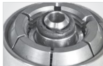
Figure 12. An example of a bad O-ring main seal
