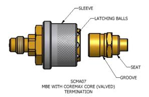
OPERATION TO CONNECT TO COREMAX SEAT: Pull the sleeve backwards to disengage the connector and insert onto the *CoreMax* seat without the *CoreMax* core. The sleeve is spring actuated, so it will move completely forward when the connector is properly engaged. Slightly pull back on the connector to insure engagement before testing. Do not pull the sleeve back after engagement.
