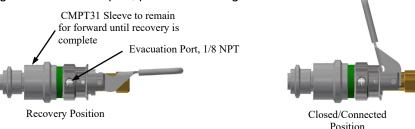
2. Once the media has been evacuated through the evacuation port, slide sleeve away from male fitting. <u>The Green Visual Indicator</u> will be covered by sleeve.
