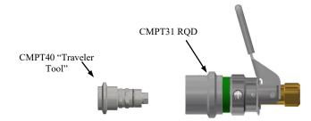
**CMPT31 RQD** Connector provides a reliable leak-tight connection that grips and seals on the CMPT40 Traveler tool. Simply insert male end of fitting and slide sleeve forward, gripping balls will secure fitting.
