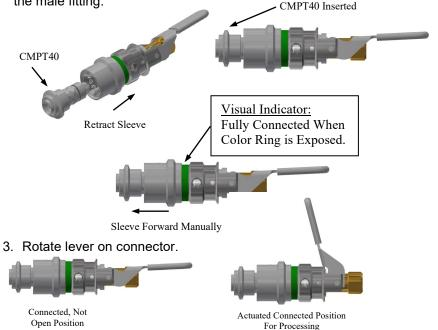
CMPT31 RQD is now sealed on the CMPT40, and valve is open for flow.
