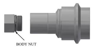
2. Remove the valve cartridge. Once the cartridge is out, the nut o-ring And valve o-ring can be removed and discarded. The new o-rings Can now be installed. Lubricate all seals with refrigerant oil.
