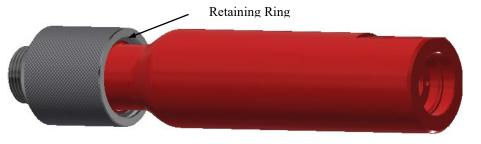
13. Insert shaft and back cap into back body and insert retaining ring in the groove to keep it in place.
